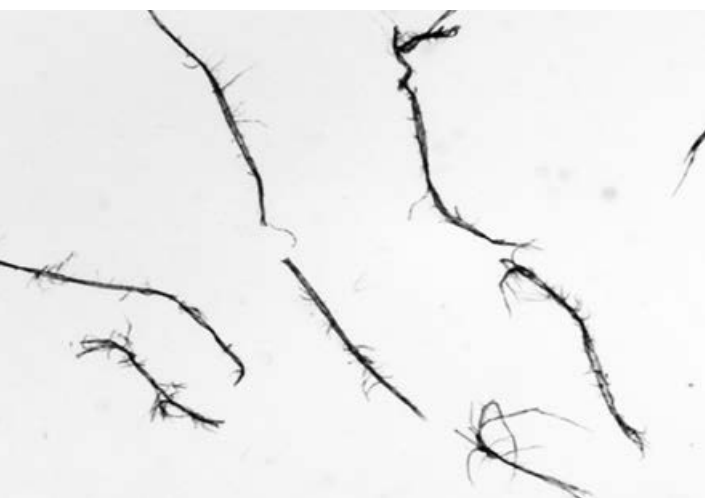
FIGURE 1 A high-definition image clearly shows fibrillation.
