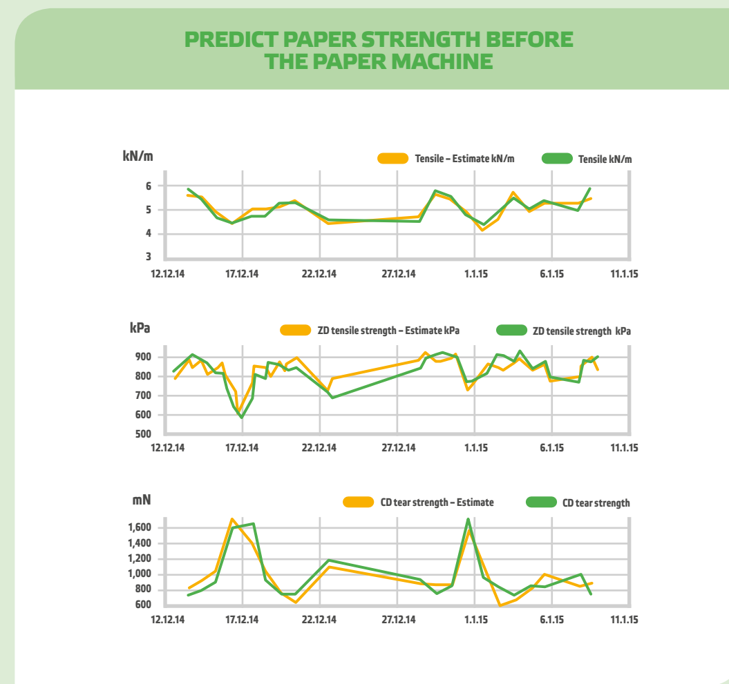
FIGURE 4 Tensile, z-direction tensile and CD tear have been predicted with models using fibrillation. Predicted values (in yellow) track lab tests (in green) very well.
