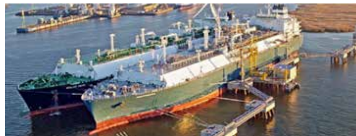
■ Fig. 5 - Floating storage & regasification unit (FSRU). Ideal for: large-size storage (from 125,000 m 3 and up), where there is at least 600 MW offtake. Advantage: a flexible solution that can be moved whenever demand changes.
