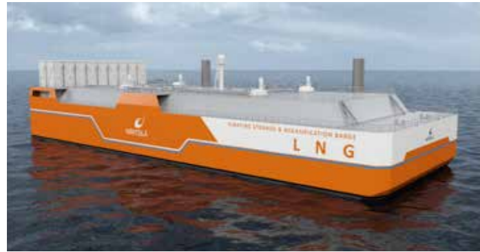
■ Fig. 2 - LNG floating storage & regasification barge (FSRB). Ideal for: locations with shallow protected water, difficult site conditions and expensive local infrastructure. Advantage: a mobile and modularised asset (in sizes from 7500 m 3 to 30,000 m 3 ) that, therefore, can be multiplied or relocated if demands change
